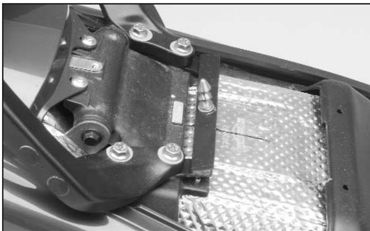
4. Use a removable strength threadlock compound (Blue Loctite for example) and tighten to 8 ft lbs.
