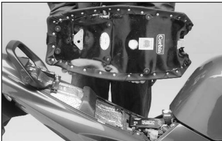
3. Remove the Triumph grab rail by taking out the four bolts shown in Figure 2. Slide the Corbin bracket into place under the grab rail and reinstall the stock bolts. If you are installing the Gunfighter model, you will NOT reinstall the grab rail and will just mount the Corbin bracket.
