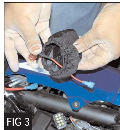
4. The fuse box cover won't close because of the fuse adapter, so close the fuse box cover loosely then cover the entire fuse box with the rain cover.
