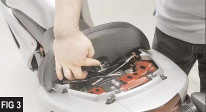
4. **Rear & Smuggler Saddle:** If you will be using the rider's backrest on the rear saddle, install it before latching seat to bike. There is a safety screw that must be installed and you cannot reach it with the seat mounted on. The rear & smuggler saddles installs with two adjustable tongues in the front and latch in the rear. Slip the front tongues under the bracket you just installed, align with rear lock and push down.
