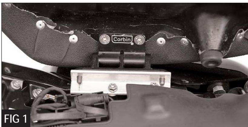
**NOTE:** Snug the bolts in place, close the saddle to get it properly aligned. Once aligned, then go back and tighten the bolts.
