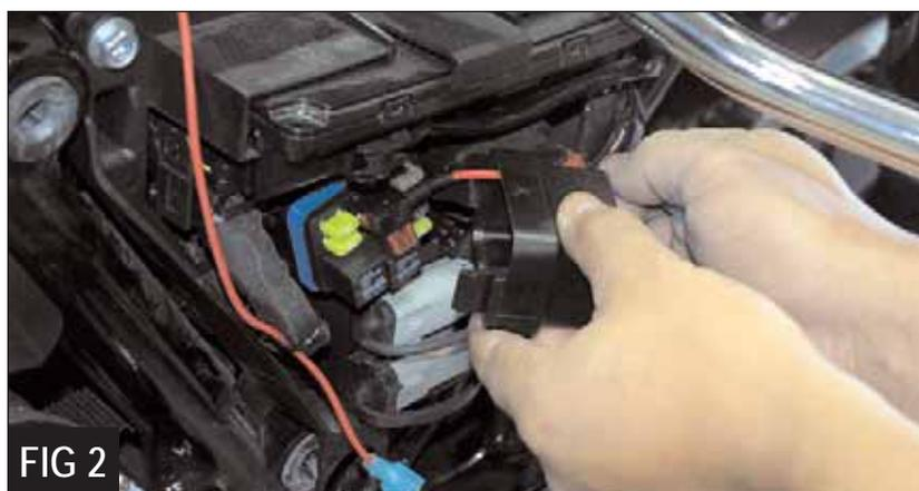
7. Drill a 3/8" hole into the top right of the fuse box cover and route the small fuse adapter wire out through the hole.
