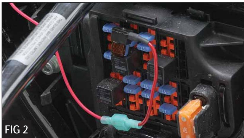
4. The fuse box is located on the left side of your motorcycle under the side cover. Open the fuse box cover and locate the Accessories fuse. Remove the Accessory fuse (check inside of fuse box cover or owners manual for it's location). Insert it into the open slot in the fuse adapter (*Figure 1*), then return it to the original accessory fuse slot in the fuse box (*Figure 2*).
