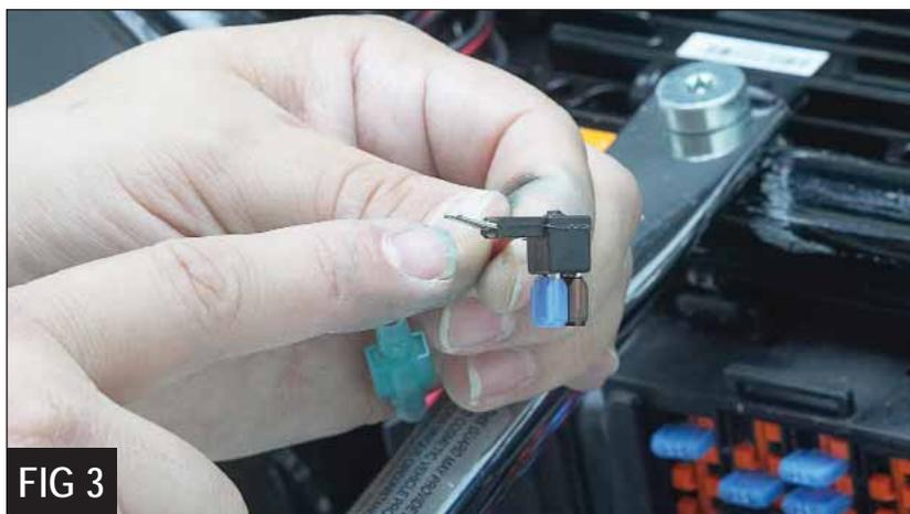
6. Route the wiring where it will not be pinched against the chassis, by the seat or other objects as this could cause a short.
