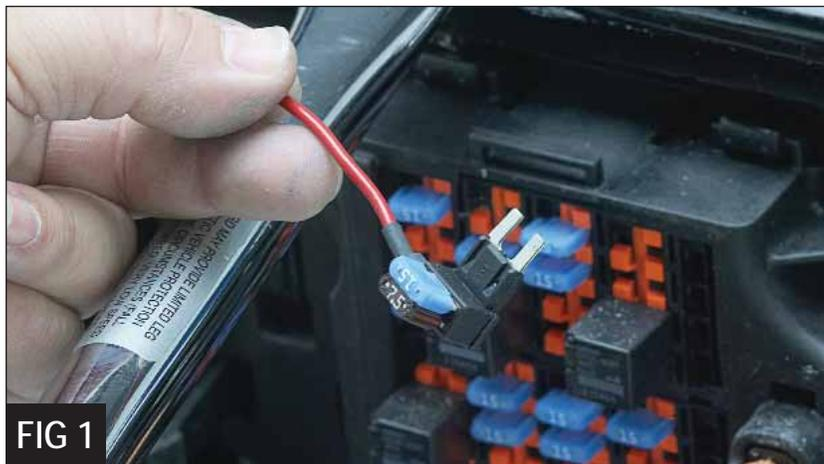
3. Installing the pigtail is simple and only requires two connections. The red wire will plug into the accessory jack of your fuse box, while the black wire connects to the ground location on the battery.
