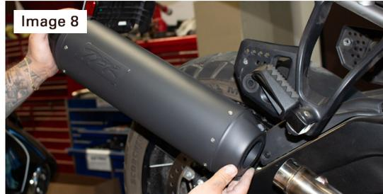
10. Slide Muffler clamp and rubber liner onto muffler. **(Reference image 9)**
