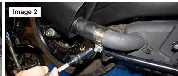
4. Remove OEM muffler support bolt. **(Reference image 3)**
