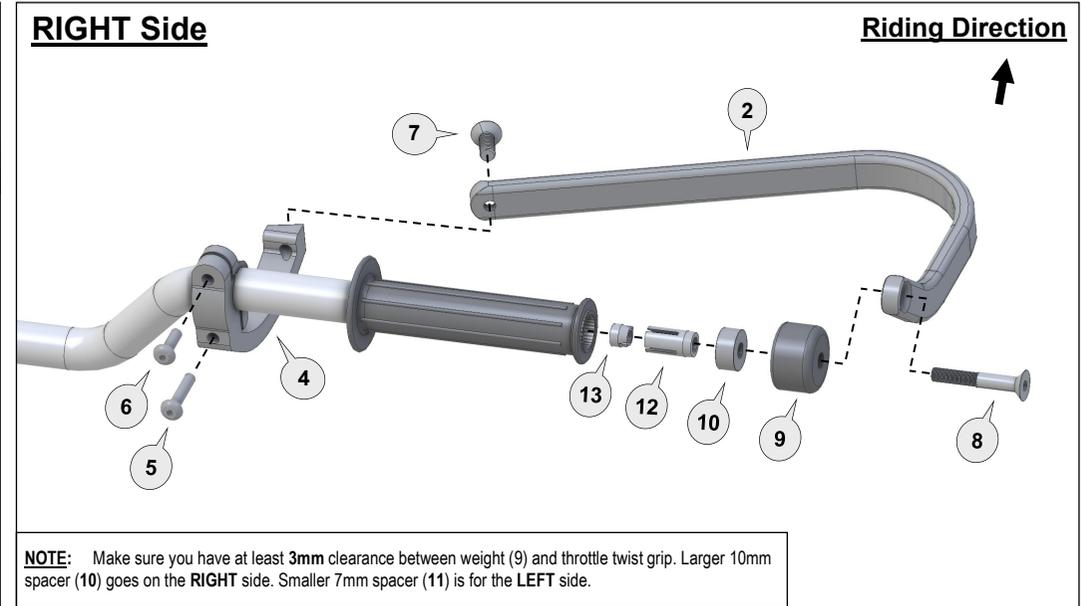
**NOTE:** Make sure you have at least 3mm clearance between weight (9) and throttle twist grip. Larger 10mm spacer (10) goes on the RIGHT side. Smaller 7mm spacer (11) is for the LEFT side.
