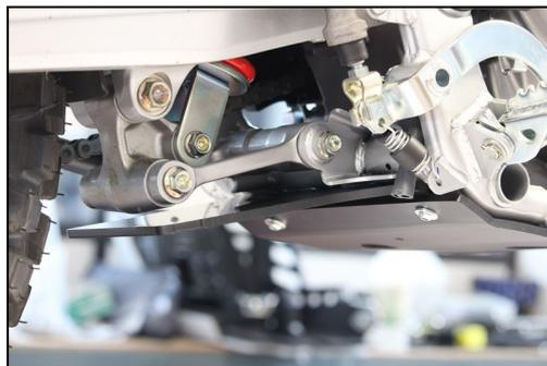
If you already have our skid plate, remove the 8mm spacers and add the linkage guard inside of the plate using the same alloy spacers and bolts.
