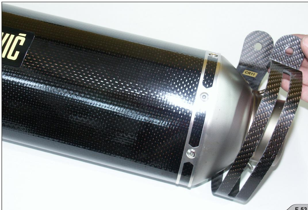
9. Position the muffler(s) correctly and slide it onto the outlet side of the link pipe(s), hand tighten the muffler clamp(s) to the bracket(s) and attach the springs
