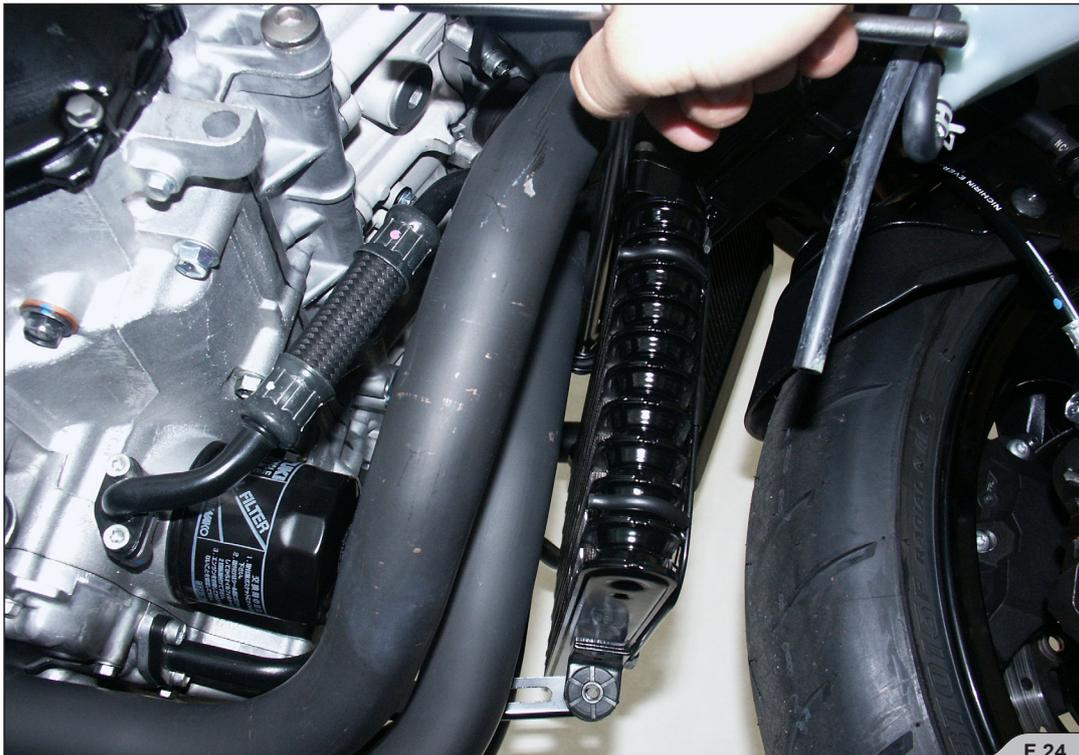
8. Unscrew the bolts from the lower oil cooler hanging bracket and remove the bracket (F 25, 26, 27). Slightly remove the cooler.
