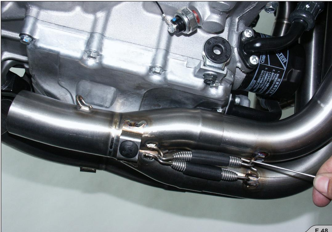
5. For Racing single exhaust only: slide the link pipe onto the collectors and attach the springs.
