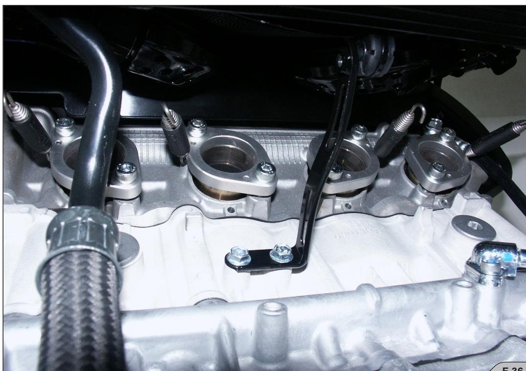
2. For easier mounting put headers together; make sure they are correctly oriented (F 37, 38, 39, 40). Insert the header tubes properly, attach the springs and tighten the flanges.
