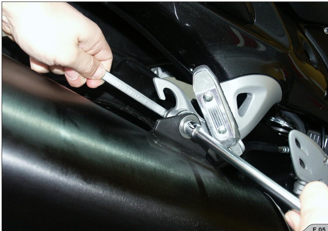
5. Remove the mufflers and the gaskets (F 06, 07, 08).
