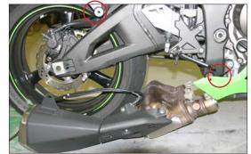
6. Remove lower right footpeg bolt and replace with supplied 8x35mm bolt.
