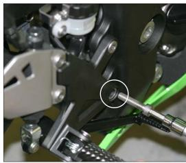
7. Install supplied mounting bracket as shown to the preinstalled supplied bolt, retain with supplied nut and 8x20mm bolt on the lower hole.
