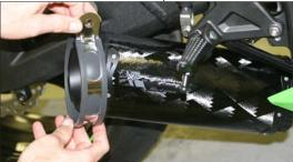
Loosely install muffler clamp to TBR bracket using the supplied 8x20mm bolt and nut.
