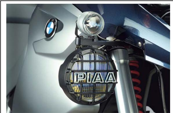
The TECHMOUNT Light Bar is designed for mounting PIAA brand driving and fog lamps as shown above. The Light Bar attaches to the small (.600") frame tube directly behind the oil cooler on a 2005 BMW R1200GS. This frame tube runs parallel to the oil cooler and provides a solid mounting location. During installation please take care not to contact the oil cooler fins as they are easily damaged. It is OK for the lower portion of the Light Bar to contact the frame of the oil cooler.
