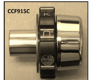
**Operation:** The friction nut has **left hand thread**. In readiness for engagement, it must be adjusted so that it makes contact with the throttle sleeve.
