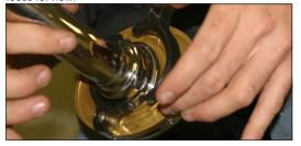
Install TBR header pipe assembly and mount muffler using the rubber lines supplied muffler clamp and secure with the supplied flange bolt, nut, and washers on each side of rubber grommit.
