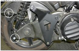
Install TBR muffler to TBR header pipe using the 6x14mm socket head cap screws and lock washers provided, leave loose for now.
