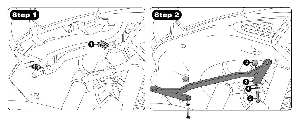
**Step One:** Remove the lower front cowl to expose the two mounting points illustrated above. Attach the supplied clip nuts onto the two mounting points. Once the clip nuts are in place, reinstall the lower front cowl to the motorcycle.
