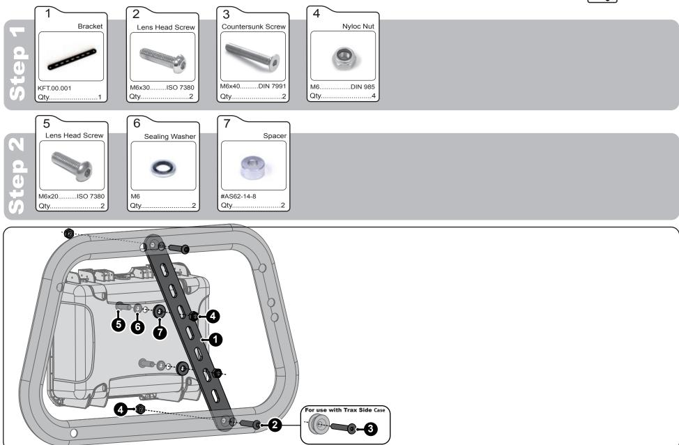
**Step One:** Bolt the mounting bracket to the rack using the included hardware. See diagram for installing with Trax Side cases.
