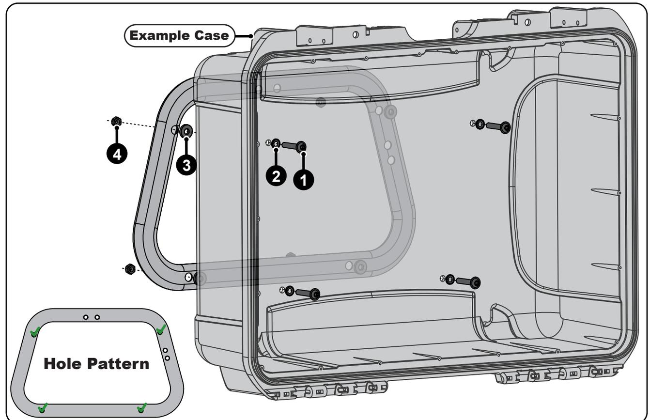
**Step One:** Place the side carrier on the back of the luggage case and mark the hole pattern on the case. Using a 6mm drill bit, drill all four holes through the back side of the case.
