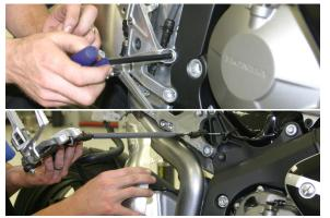
12. Loosen the OEM barrel clamp connecting the exhaust tube and header.
