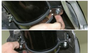
25. Securely tighten barrel clamp.
