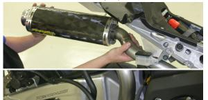
Slip upper & lower halves of muffler clamp onto muffler canister and attach to "L" brackets using supplied 8mm nuts and 8mm bolts.
