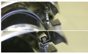
24. Making sure that the muffler canister is aligned correctly, securely tighten the 8mm bolts connecting the muffler clamp halves to the "L" brackets.
